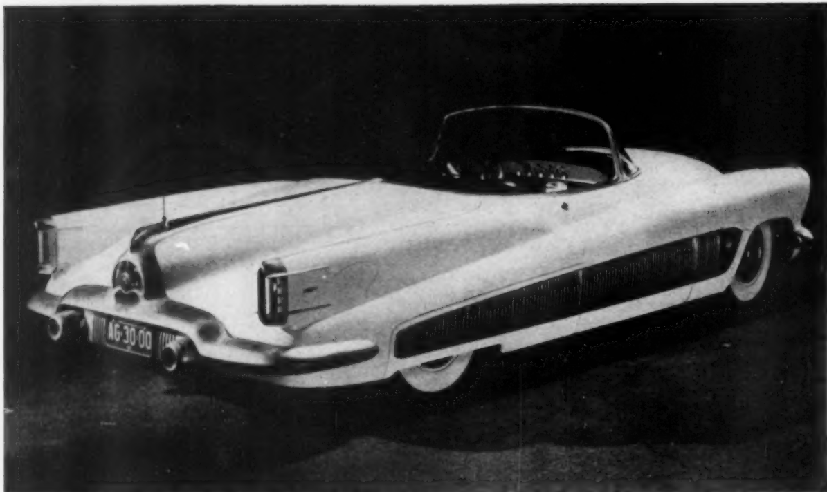
New Convertible features 335 h.p. V-8 engine, a removable top, adjustable steering wheel, and built-in hydraulic jacks.
